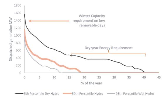
• More than 750MW of peaking capacity is required in less than 1% of hours in typical hydrology (50th percentile) to maintain security of supply.
